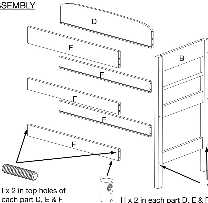
The dowel nuts (parts H) fit into the holes in the undersides of parts D, E and F. The slot on one end of the nut indicates the direction of the threaded hole and should be visible when the nut is inserted. It is advisable to push each nut into its hole and check for correct alignment before inserting any screws.
