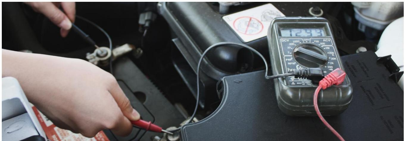
2.) Take a voltage reading with a voltmeter.
