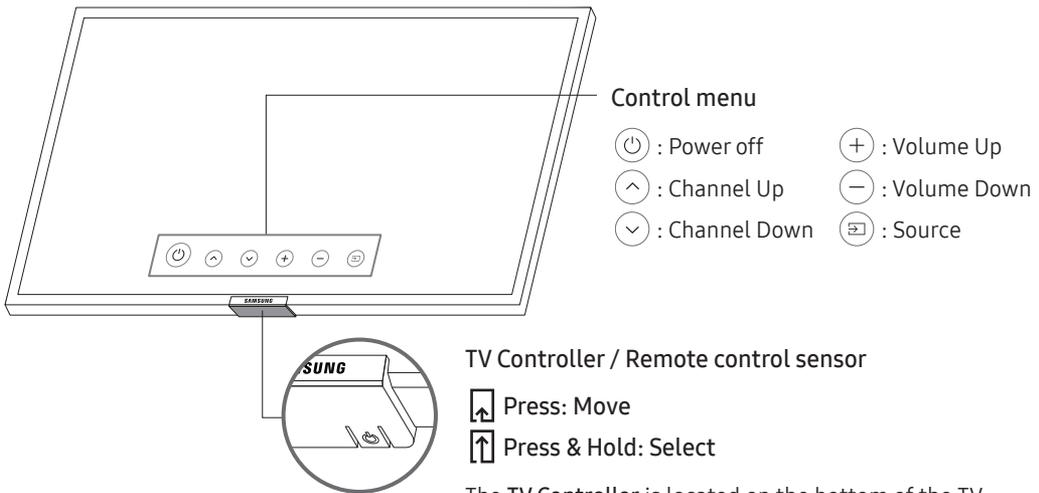
The TV Controller is located on the bottom of the TV.
