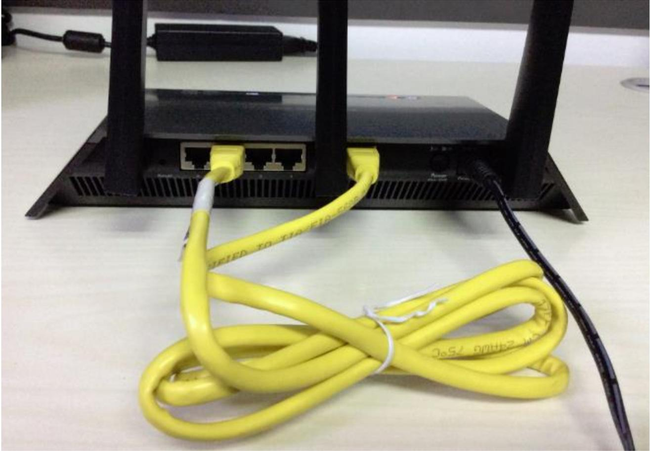
4. Check the LEDs. The LAN LED and WAN LED should both be lit. In this example, LAN 3 LED and WAN LED are both lit.
