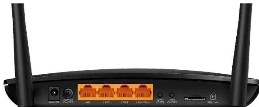
2. Press the WPS button of the client device within two minutes.
