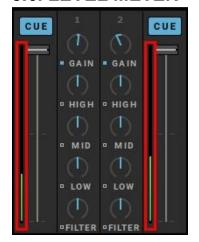
Level meters show the volume before the volume fader. Adjust the GAIN to change the volume before the volume fader.
