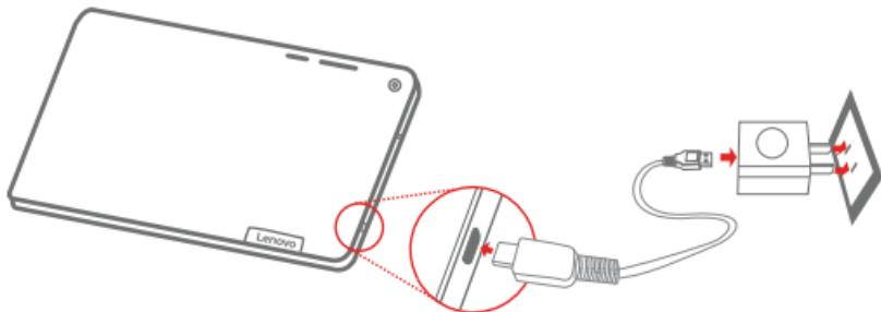
Connect your tablet to a power outlet using the included cable and USB power adapter.
