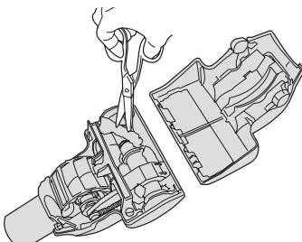
Using a pair of scissors, cut any hair or debris free from around the brushes.
