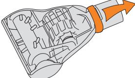
Turn the TurboTool over and slide off the locking ring.
