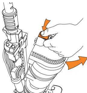
Press the dirt container release button and pull to remove the dirt container.
