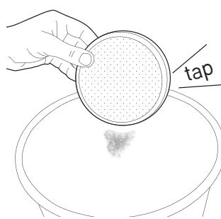
Tap the filter over a bin to release any dirt.
