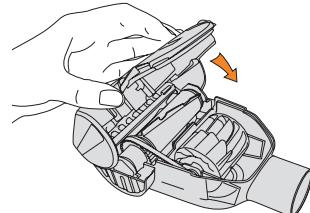
To re-assemble the TurboTool, ensure that the tabs are engaged and pivot the lower housing closed. Slip the locking ring over the neck of the TurboTool and into the groove to finish.
