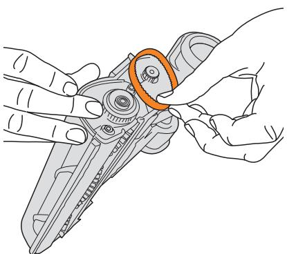
Replace the old belt, ensuring the teeth are fully engaged with the cogs.
