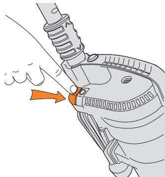
Plug in your machine and push ON/OFF button to switch on.
