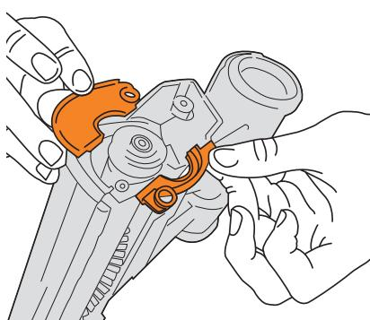
Replace the old belt, ensuring the teeth are fully engaged with the cogs.
