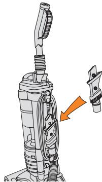
Place the 3-in-1 tool onto the on board storage area.
