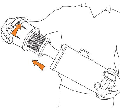
Turn the dirt container lid anti-clockwise and lift to remove.
