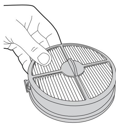
Check the post-motor filter for discolouration.
