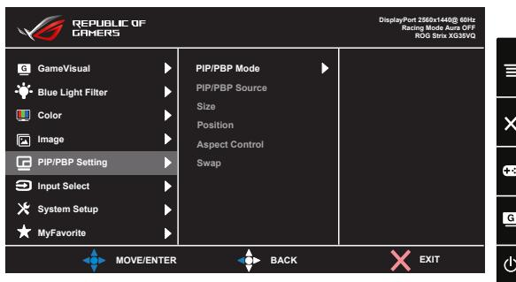
By activating this function, this monitor displays two pictures from two different video sources.
