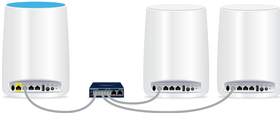
Figure 15. Ethernet backhaul connection using a switch
