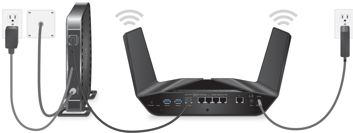
Figure 6. Cable your router
