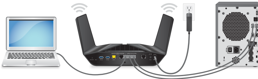
Figure 7. Ethernet port aggregation
