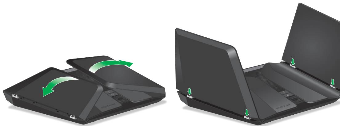
Figure 4. Position the antennas
