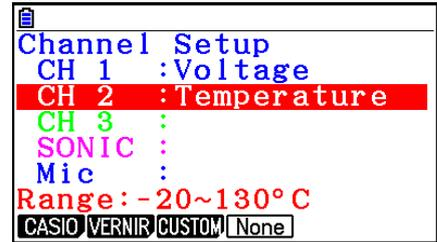
In the above example, the range of the temperature sensor assigned to CH2 appears on the display.
