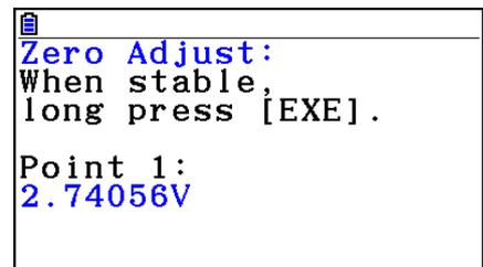
4. At the point your want to perform zero adjustment (the point that the displayed value is the appropriate zero adjust value), press **EXE**.
