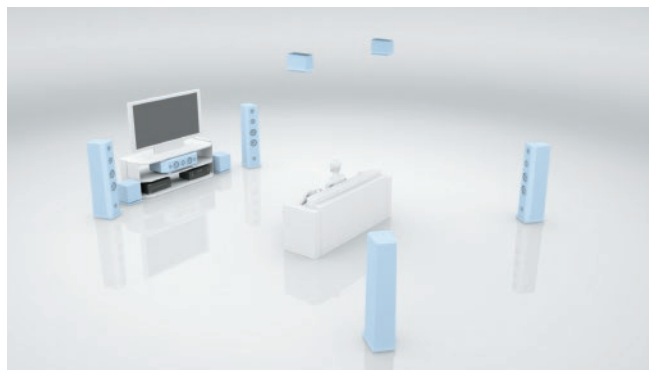
Speaker Layout Example of a Dolby Atmos Home Cinema (5.2.2ch)
