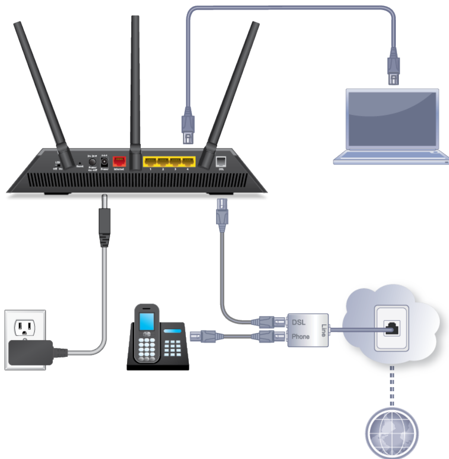
Figure 6. Modem router cabling for DSL service
