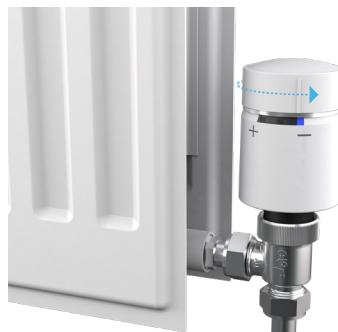
Twist the cap in the - direction and hold for 2 seconds until the blue LED lights up.
