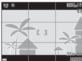
**3** Press the shutter-release button all the way, and then remove your finger from the shutter-release button.
