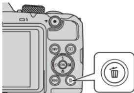
2 Use the multi selector
