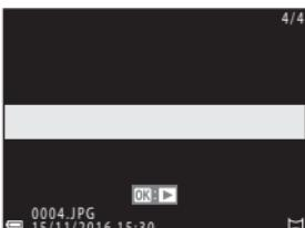
Playback controls are displayed on the screen during playback. Use the multi selector **◀▶** to select a control, and then press the **OK** button to perform the operations described below.
